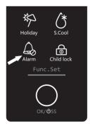
DOOR ALARM: if you leave door open over 60 seconds, the anomalous condition will be notified by intermittent buzzer. The alarm condition will stop closing the door or manually by pressing key B to select alarm function c and press key C, but in this second case alarm condition will restart after 30 seconds if door is still open.
